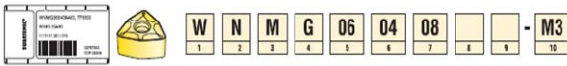
Fig. 5 Inserts coding: 1 - shape of removable insert; 2 - rake angle; 3 -tolerance; 4 - type; 5 - length of cutting edge; 6 - thickness; 7 - tip radius; 8 - edge direction; 9 - version; 10 - description (for rough cutting R, for medium M and for finishing F).
