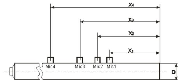
Fig. 1 Positioning of the microphone [1], [2]
