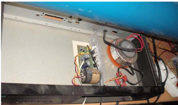
Fig. 5 Audio-frequency amplifier
