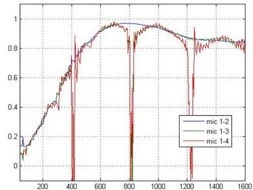
Fig. 15 Mediated absorption coefficient for the 3 measured in the range of 40-1500 Hz frequency, carried out with sample
