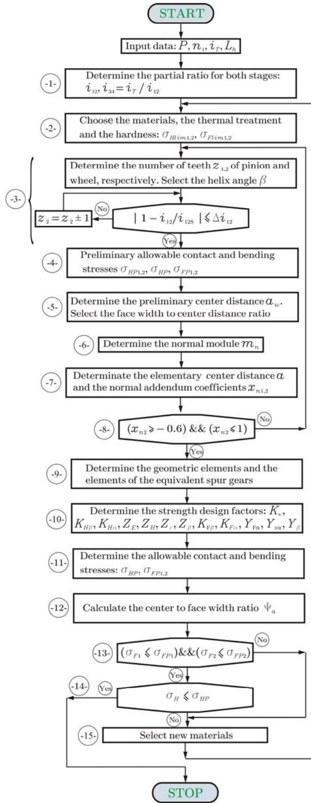
Fig. 1. The flowchart of traditional helical gear design
