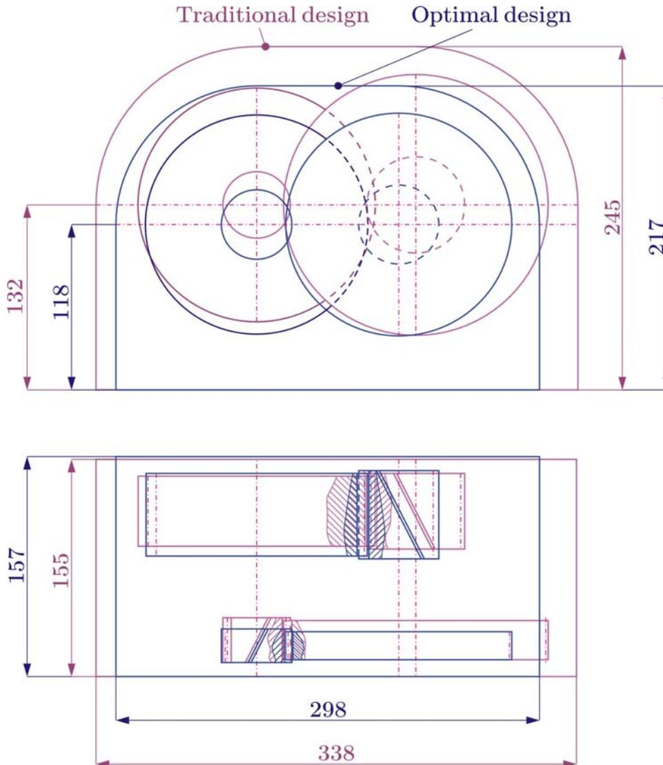
**Fig. 3.** Traditional and optimal design solutions.
