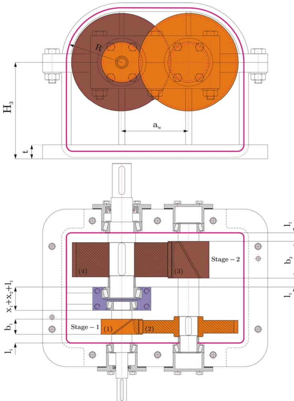
Fig. 2. The sketch of the 2 stage coaxial helical speed reducer
