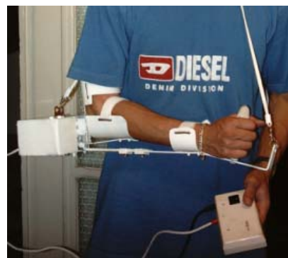
Fig. 3. Wearable exerciser for passive forearm pronation-supination
