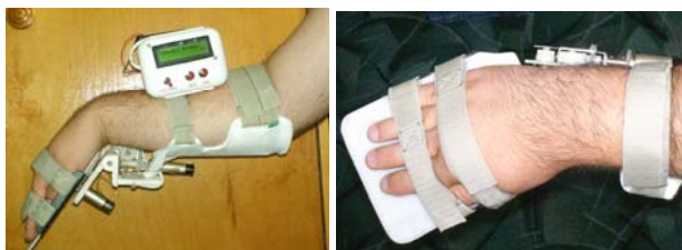
Fig. 5. Wearable wrist robotic exerciser – the first variant
