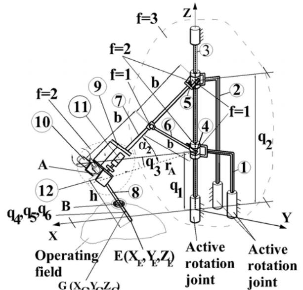
Fig. 3. The kinematic scheme of hybrid parallel robot
