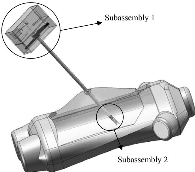
**Fig. 5.** PARASIM active surgical instrument
