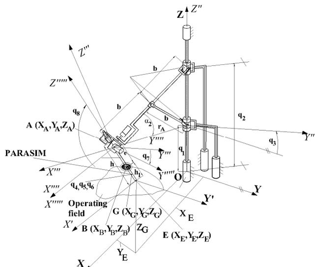
Fig. 2. Structural construction of PARASURG-9M
