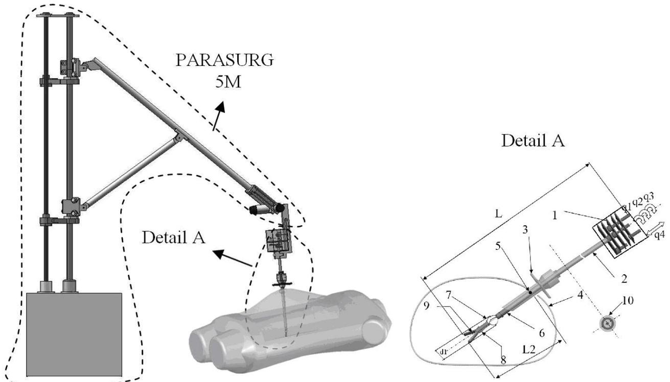
Fig. 1. a) The surgical robot PARASURG 9M, b) detail A: the active parallel robotic instrument PARASIM
