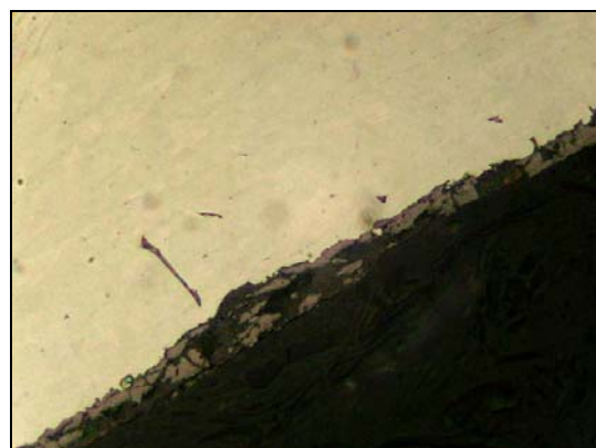
Figure 7. WC -Co powders prayed onto steel plate
