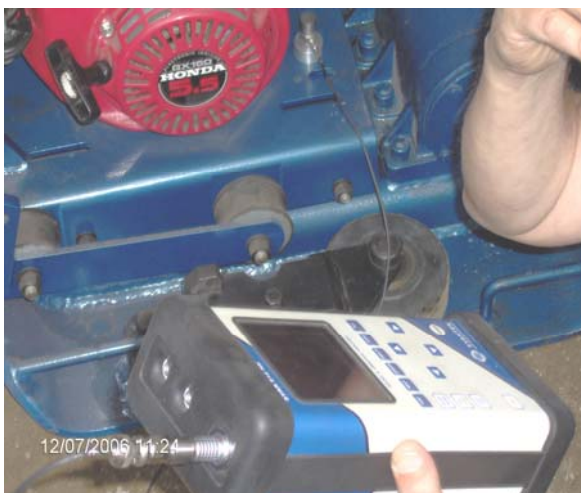
Fig. 4. The measurement of vibration at the level of plate compactor's components
