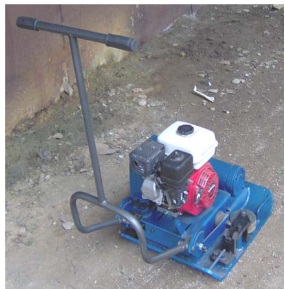
Fig. 3. The plate compactor
