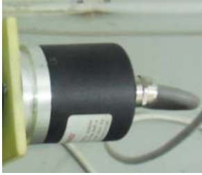
Fig. 2. Rotary incremental sensor EA44
