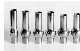
Fig. 2 Parts with walls reaching breaking point during hydroforming process
