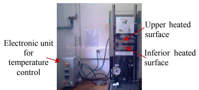
Fig. 2 Compression moulding machine used to form the test bars.
