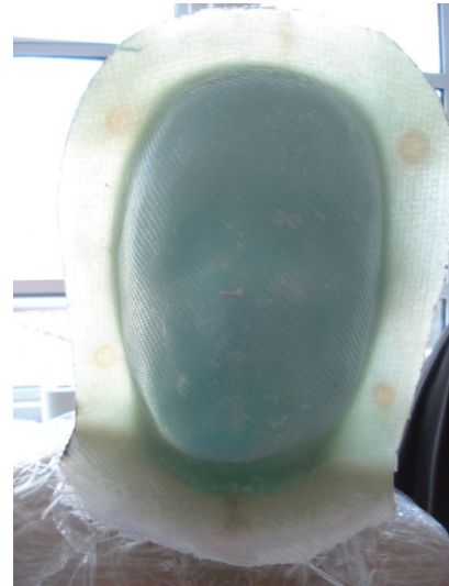
Fig. 6. The glass fiber reinforced epoxy mold
