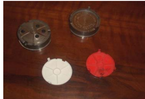
Fig. 6. SLS Prototype, tools and injected part measured on Zeiss Eclipse CMM
