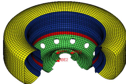
Fig. 3. The wheel mesh layout
