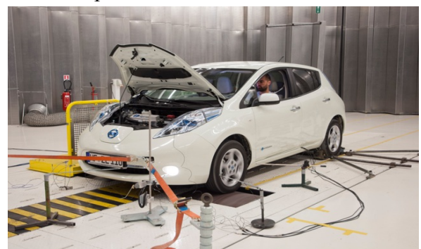
Figure 1. Electric car testing on the chassis dyno inside an semi anechoic chamber
