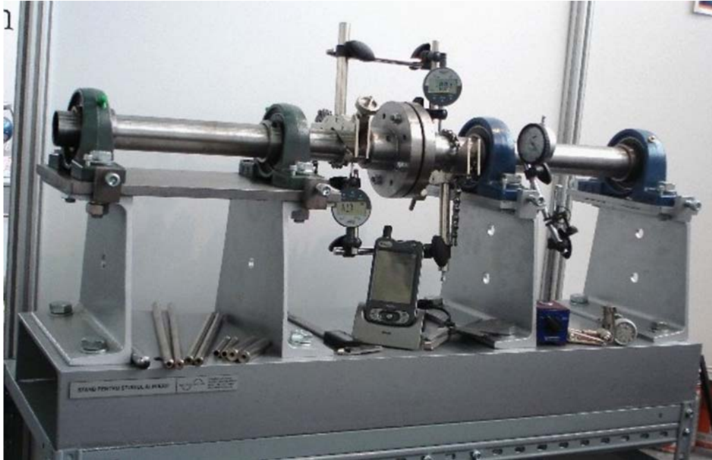
Fig. 5. Stand for horizontal shaft alignment study
