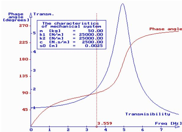
Fig. 13 Transmissibility and phase angle (Zener model)
