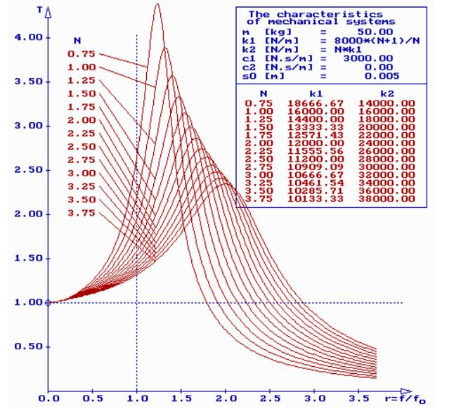
Fig. 12 The transmissibility diagrams ( $c_1 = 3000$ )
