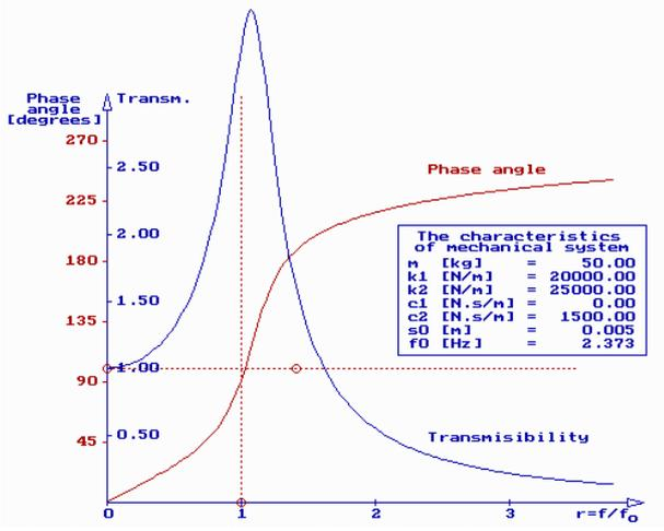
Fig. 8 Diagrams of transmissibility and phase angle for specified numerical values
