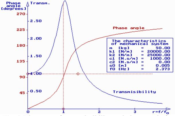
Fig. 9 Diagrams of transmissibility and phase angle for specified numerical values
