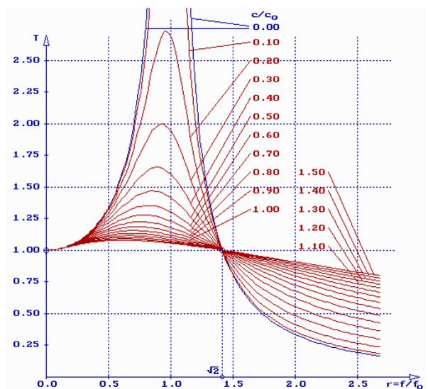
Fig. 1 The transmissibility diagrams [15]
