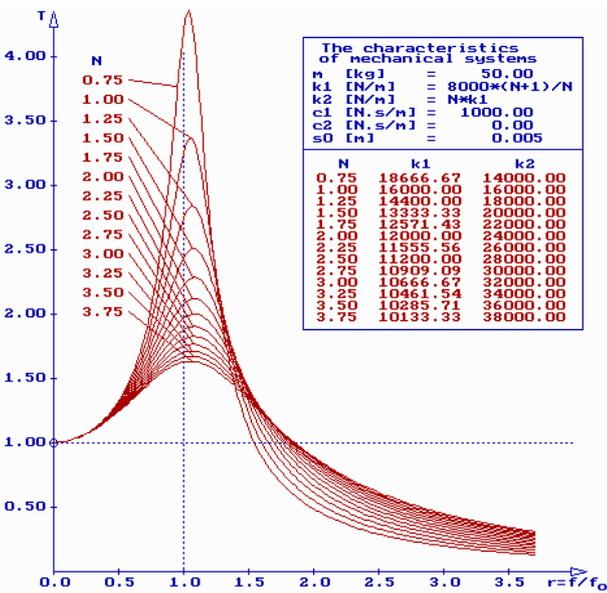
Fig.10 The transmissibility diagrams ( $c_1 = 1000$ )
