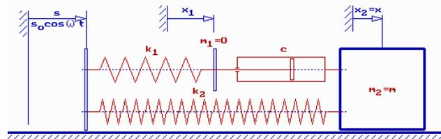
Fig. 6. The mechanical system containing the Zener's rheological model
