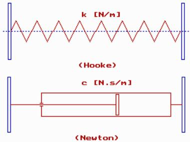
Fig. 2. The Hooke's and Newton's elements
