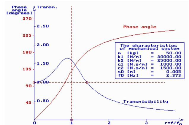
Fig. 7 Diagrams of transmissibility and phase angle for specified numerical values
