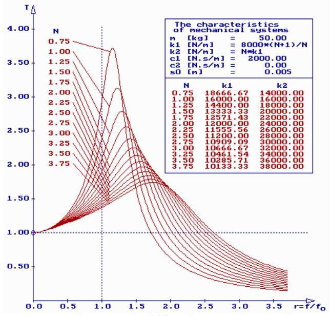
Fig. 11 The transmissibility diagrams ( $c_1 = 2000$ )
