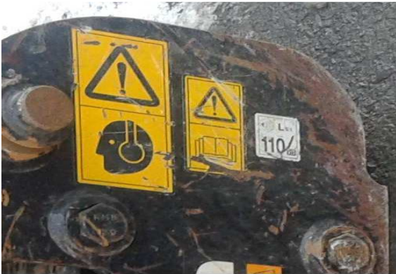
Fig. 4. Sound pressure marking of pneumatic hammer
