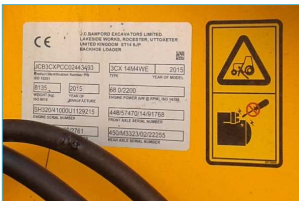
Fig. 5. CE marking on the excavator
