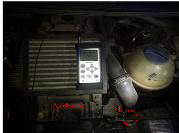
Fig. 2. Location vibration measuring system for P1 measurement point.
