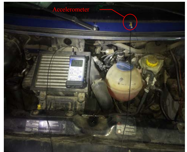
Fig. 5. Location vibration measuring system for P2 measurement point.
