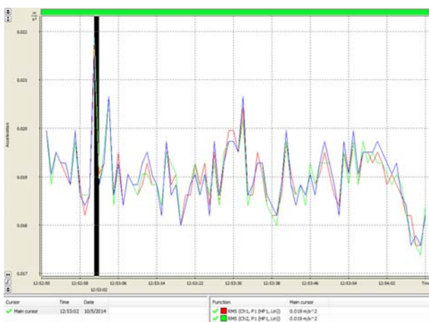
Fig. 5. Oscillogram of RMS acceleration from the P1 measuring point.
