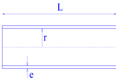
Fig.2 Tube under external pressure
