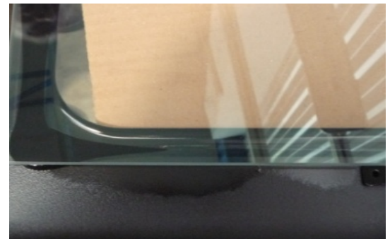
Fig.20. Application of patchy thickness of the adhesive
