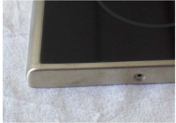
Fig.14. The metallic support made of stainless steel sheet and assembled by bonding with ceramic glass.
