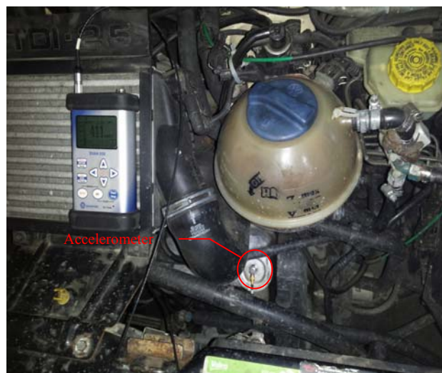
Fig. 3. Location vibration measuring system for P1 measurement point.
