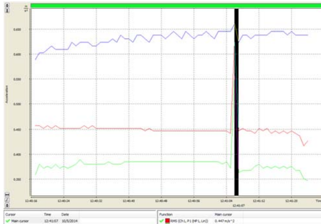
Fig. 10. Oscillogram of RMS acceleration from the P3 measuring point.
