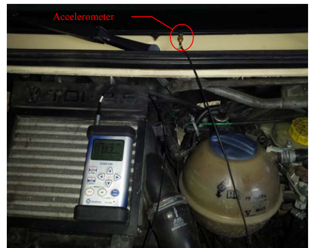
Fig. 6. Location vibration measuring system for P2 measurement point.
