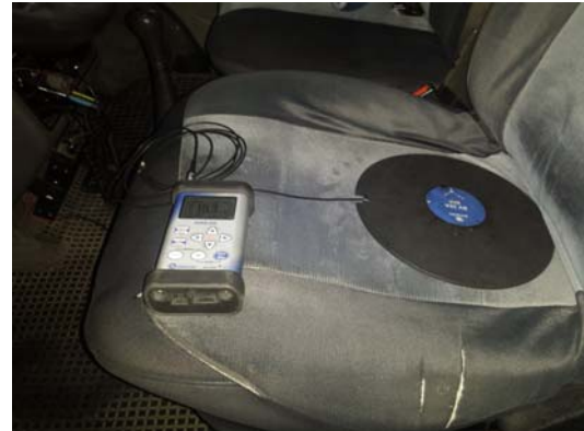
Fig. 8. Location vibration measuring system for P3 measurement point.
